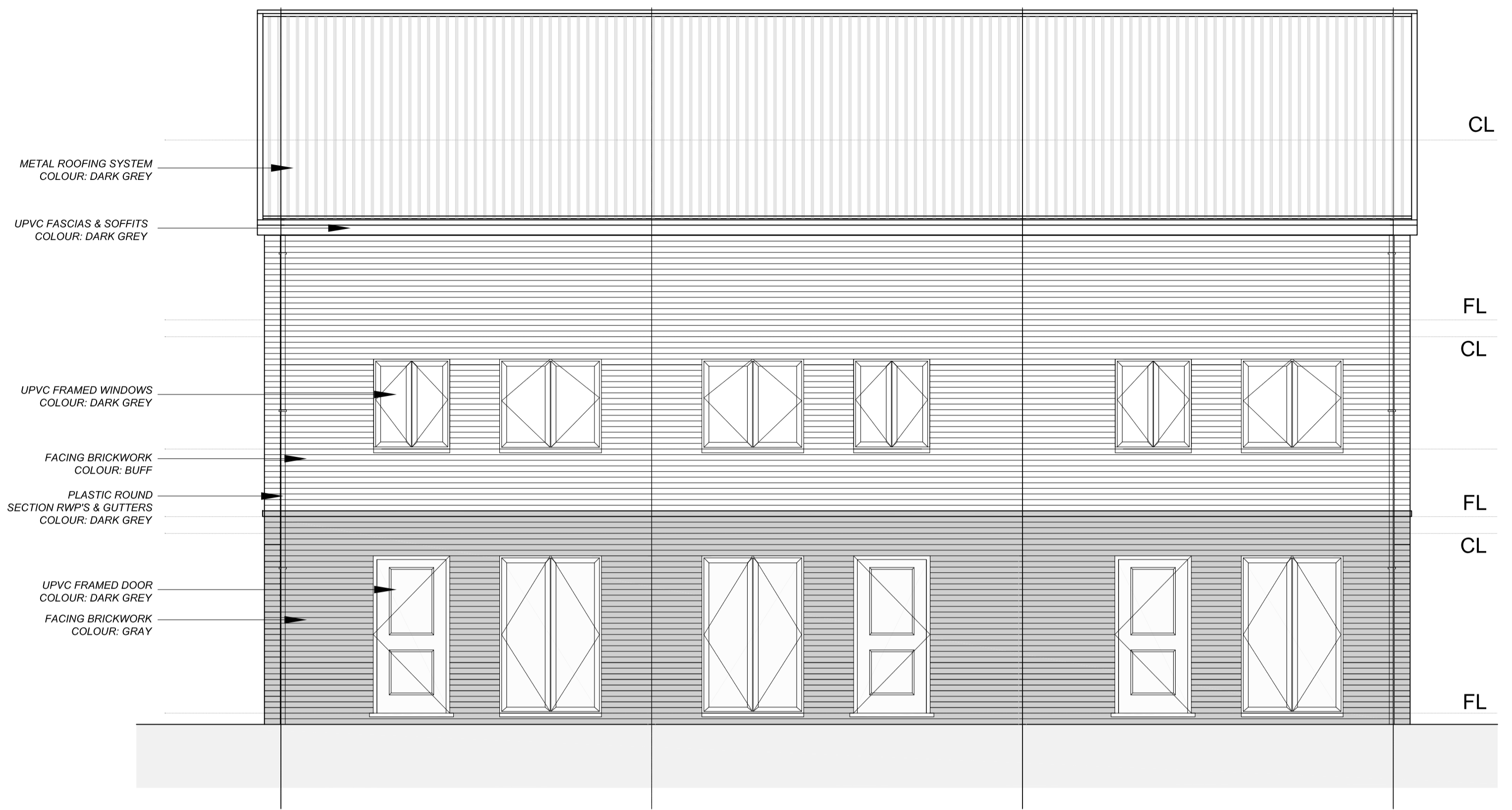
PROPOSED SOUTH ELEVATION
